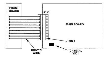
Figure 4-1. Front Subassembly Installation
